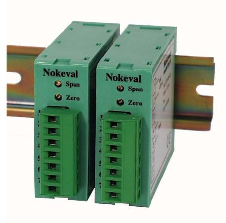
Loop powered galvanic accuracy isolator 6570 is designed for current input 4..20 mA works without auxiliary operating voltage. Converter is serial connected into a current loop which will be galvanic isolated over to the output 0..20 mA, 4..20 mA or 0..10 V. Typical inaccuracy is smaller than 0.05% of full scale.
