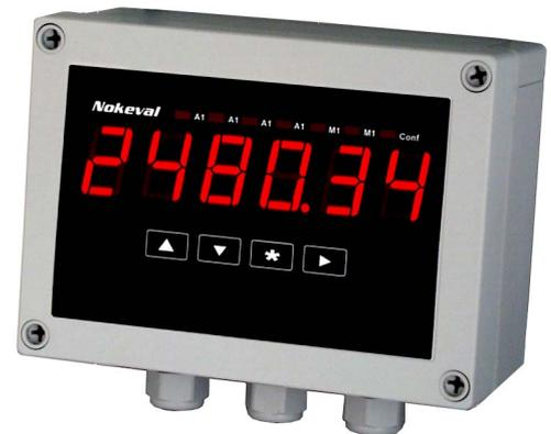
The field display 2071 is designed for serial communication. It uses the simple Nokeval SCL protocol where only the address, value and check sum are sent. The display has both the serial inputs RS-232 and RS-485 as a standard. The serial bus is galvanically isolated from the processor and the power supply. In the configuration mode you can set the address, baud rate and the type of number value that you want to appear on the display after power connection.
