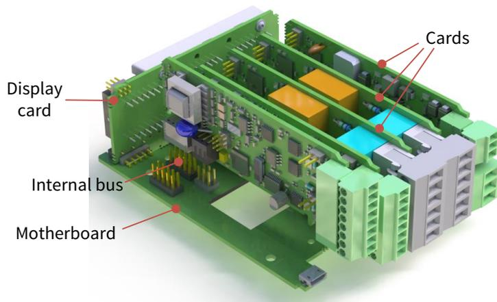
The cards are printed circuit boards without an enclosure of their own. The desired types of cards are inserted on the motherboard.
