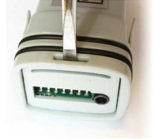
When the cover plate is removed, the circuit board can be pulled out of the enclosure.
