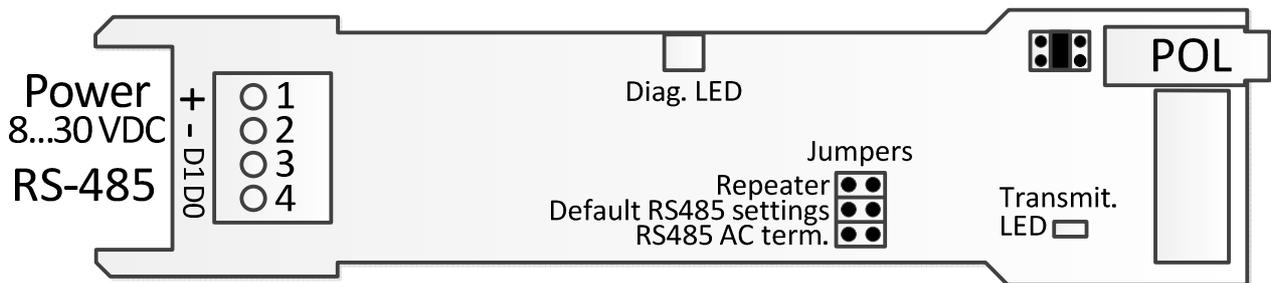
FT20 serial module has a 4-pin terminal block for power supply and RS-485 connection. Serial module features also a round 3.5 mm POL programming connector jack found on many other Nokeval products as well. FT20 radio module contains BNC type antenna connector.
