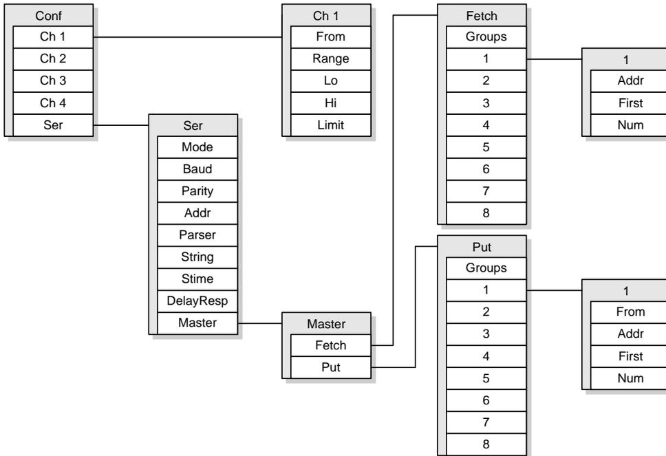
The menu is arranged hierarchically. The first level contains four submenus, one for each analog output, and a serial communications submenu. Some of the settings are hidden when they are not used.
