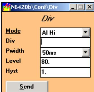
Pulse output and alarm settings by MekuWin software.
