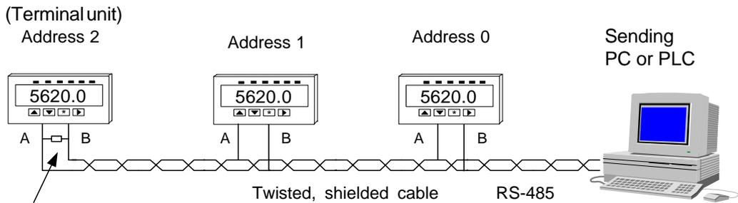
Terminal resistor (110 ohm) in last unit (Jumper J2 on)
