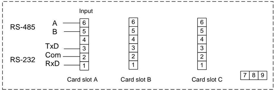
Only one of the serial connectors can be used at a time.
