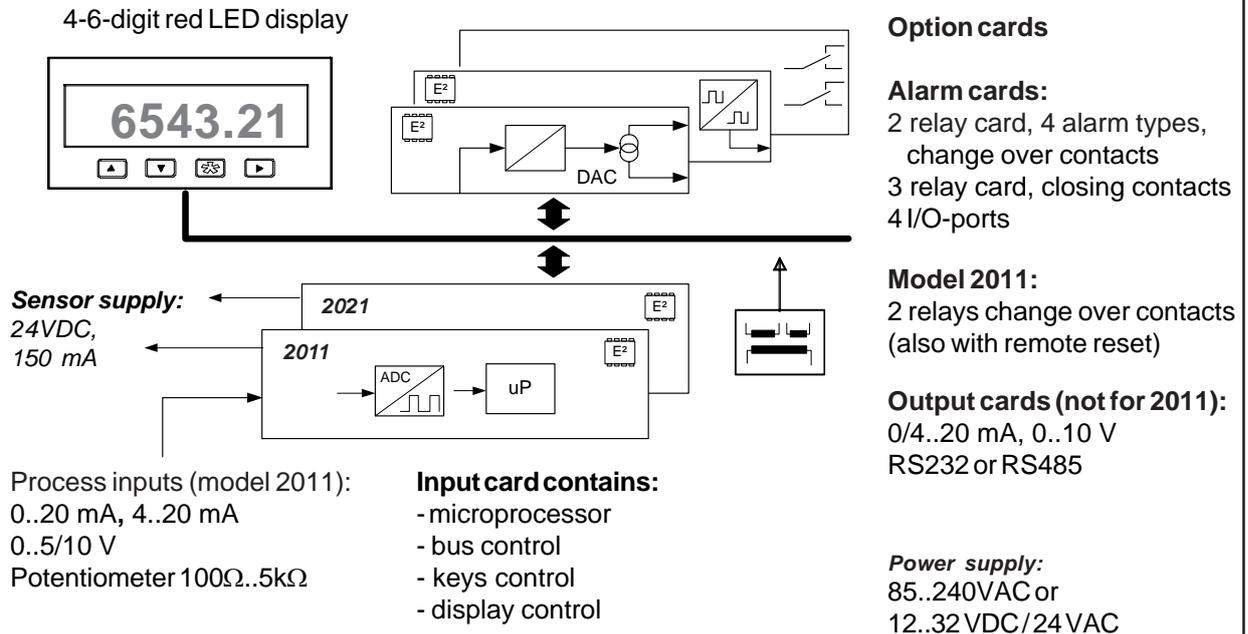
Model 2021 contains also process inputs but it can also measure RTD-sensors and thermocouples. 2021 has very accurate and fast A/D-converter (16 bit 1/64 000).
