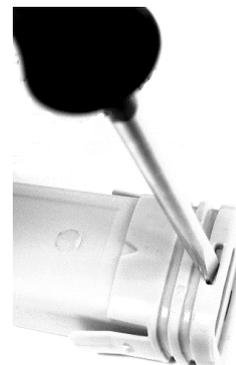
Assemble reversely, taking care that the circuit board sits on the grooves.
