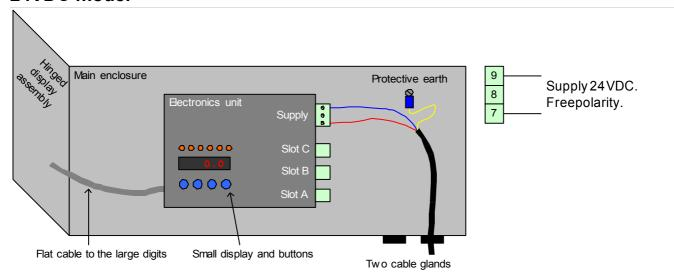
Bring the supply voltage to the connector indicated in the picture. A pre-fuse is not necessary, but if one is used, it should be at least 2 AT. The protective earth is not required for electrical safety, but will protect from EMI fields.
