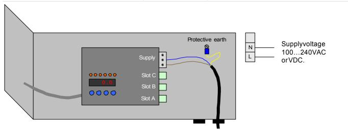
Bring the Live and Neutral wires to the electronics unit as in picture. Connect the Protective Earth wire to the M4 screw using the Faston connector provided - a Faston crimping tool is needed. A pre-fuse is not necessary, but if one is used, it should be at least 500mAT.
