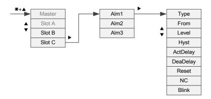
There are two or three identical submenus, corresponding to two or three relays.
