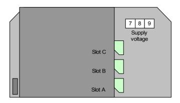
In the 24VDC model the power supply is connected in the base card terminals 7 and 9. The polarity does not matter. The connector is green.
