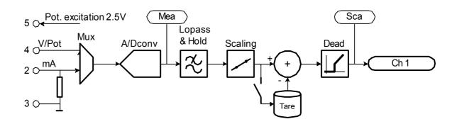
The microcontroller sets the multiplexer "Mux" to measure the V or mA input
