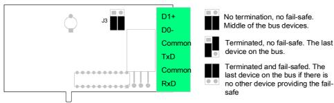
The serial communications card 2000-RS works most often with the factory set jumpers: no termination. But if the RS-485 bus is long (>50 m), the last device on the bus should be terminated.
