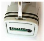
When the cover plate is removed, the circuit board can be pulled out of the enclosure.
