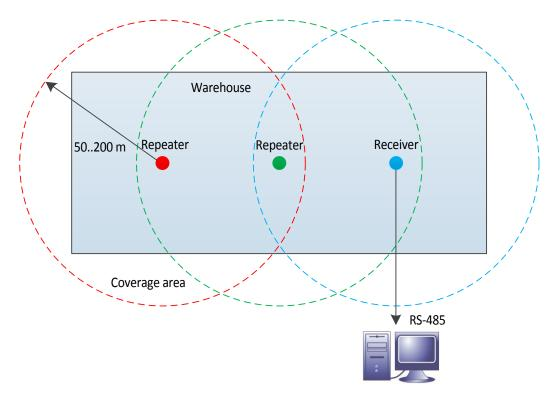
The downside of daisy chaining is that now both repeaters relay also the data that they receive from the other repeater. This increases radio traffic and therefore decreases the maximum allowed number of radio transmitters in a coverage area. See the transmitter's manual or example table on page 6 how the use of repeaters affects the maximum number of transmitters.
