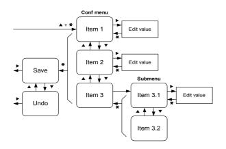
The menu is organizated hierarchically. You can enter General, Input, Output, Alarms, and Serial submenus by selecting them with  $\blacktriangle \forall$  keys, and entering the submenu with  $\triangleright$  key. See the menu chart in chapter Settings.
