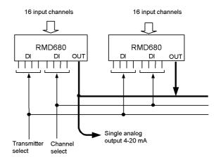
The other way is to select address 1 in every transmitter and connect a enable line to every transmitter connector K5. Bringing a voltage to this terminal activates the output.
