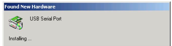
Install VirtualSerialPort-Driver same way as USB-driver. OK-LED of converter should turn ON.
