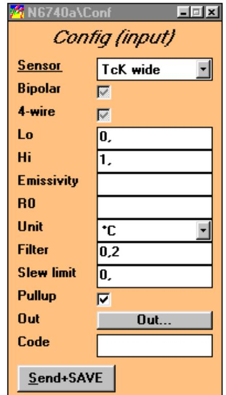
Typical settings for K-type thermocouple
