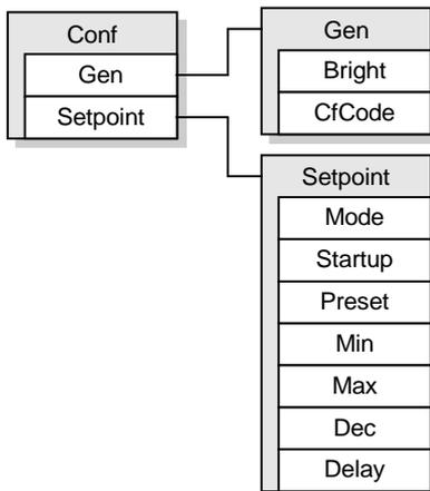
The configuration menu of the master is divided in two sections, Gen (general) and Setpoint settings.
