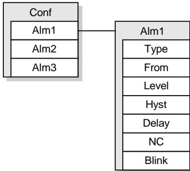
The configuration menu has two or three submenus, depending on the card type. The submenus are identical.
