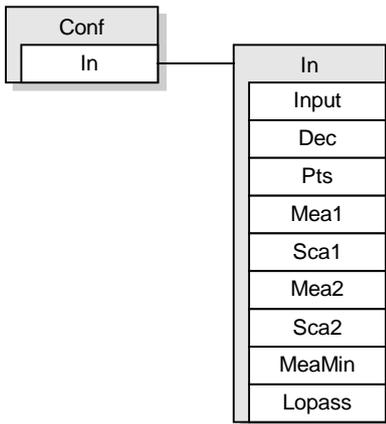
The configuration menu has one submenu, In, that contains the input settings.
