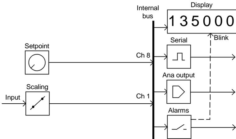
The mA or V input is first measured. This information is converted to a scaled reading (in any engineering units) using two freely selectable sample points, e.g. 4.112 mA corresponds to 0 bar and 16.501 mA corresponds to 6 bar. This is set up in slot A configuration menu. The reading is put available on internal channel 1, to be available for the outputs and the display.
