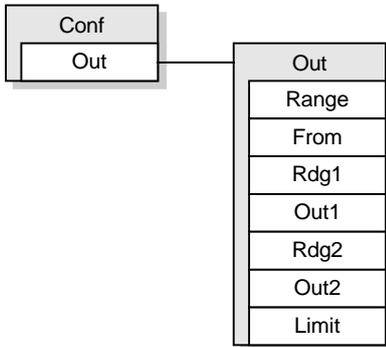
All the output settings are in submenu Out.
