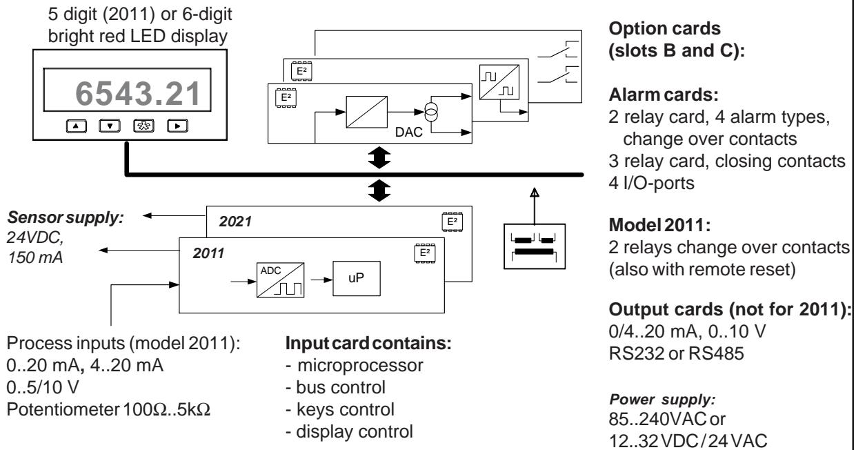
Model 2021 contains also process inputs but it can measure RTD-sensors and thermocouples. 2021 has very accurate and fast A/D-converter (16 bit 1/64 000).
