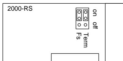
When using serial signal RS485 last unit must be terminated 110 ohm resistor. You can make termination at terminal connectors or connecting jumper J1 to ON position.
