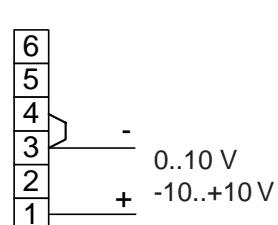
0..10 V input requires moving jumper J1 to position 1-2, for other inputs select 2-3.
