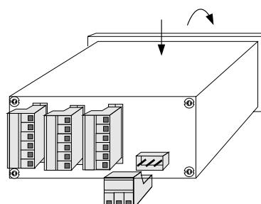
Press gently case behind front panel and draw frame outwards gripping upper part of frame.
