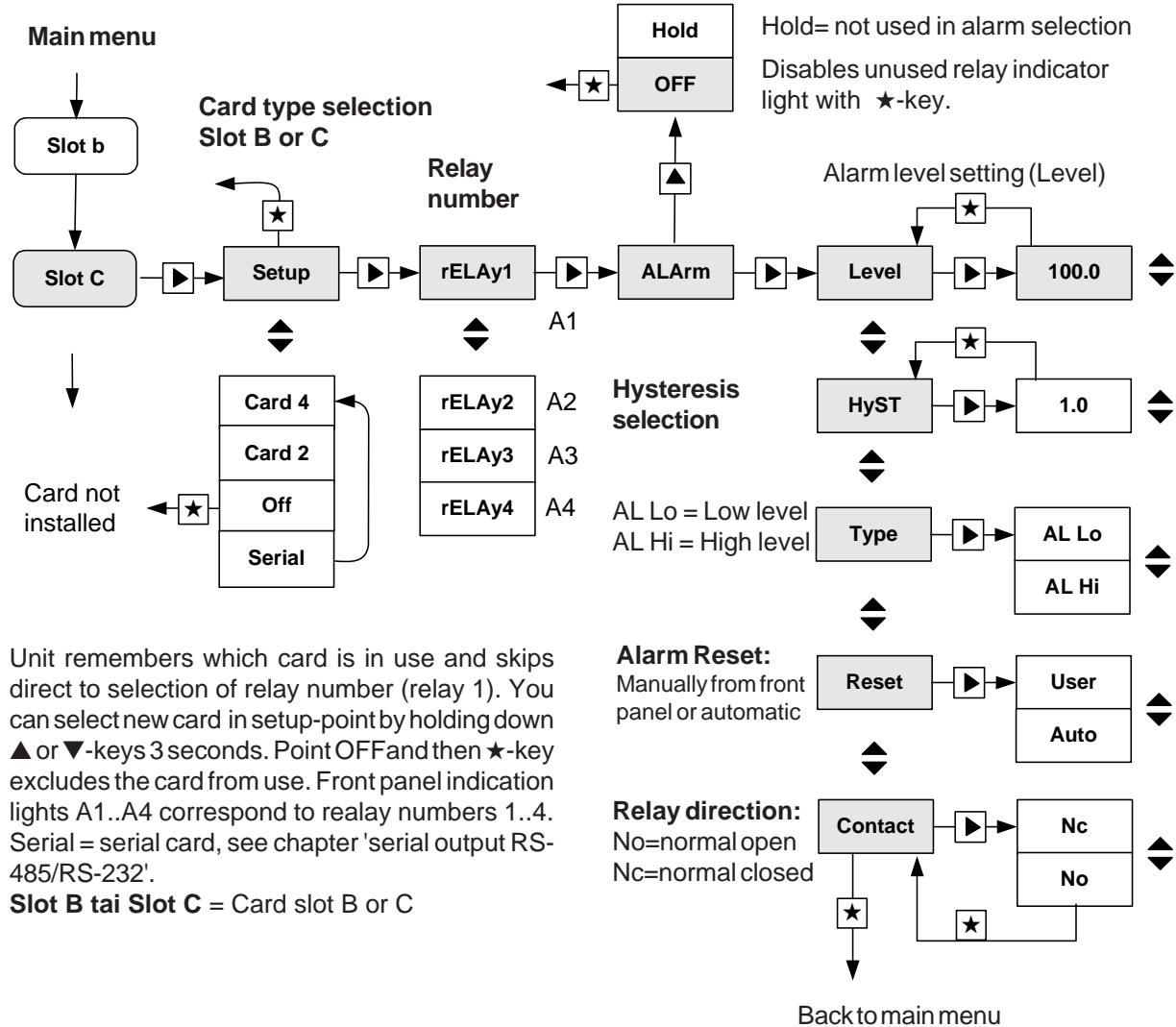
Unit remembers which card is in use and skips direct to selection of relay number (relay 1). You can select new card in setup-point by holding down ▲ or ▼-keys 3 seconds. Point OFF and then ★-key excludes the card from use. Front panel indication lights A1..A4 correspond to realay numbers 1..4. Serial = serial card, see chapter 'serial output RS-485/RS-232'.
