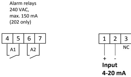
Models 301 and 302: connectors are located inside the device behind the display.
