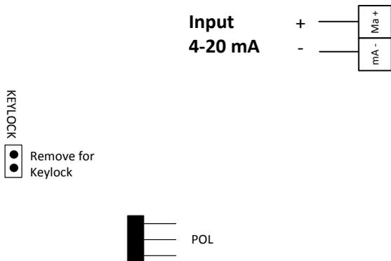
Connect the 4...20mA input to terminals 1 (+) and 2 (-). On models 301/302/305, refer to the polarity markings on the circuit board.
