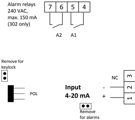
Model 305: connectors are located inside the device behind the display.
