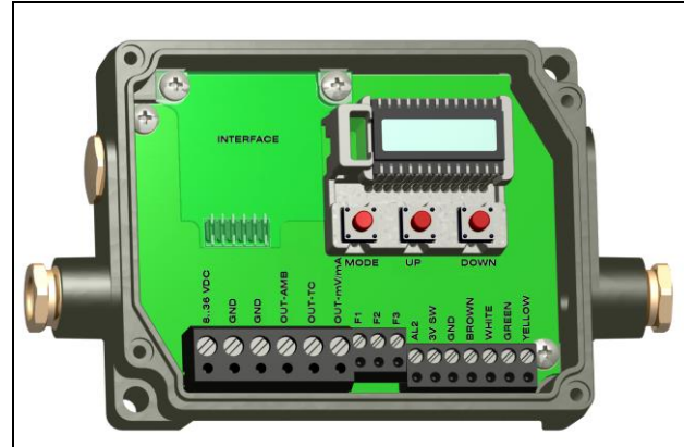
Figure 14: Opened electronic box (LT/ LTF/ MT/ F2/ F6/ G5/ G7/ P7) with terminal connections
